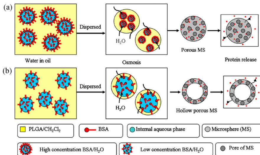
Fig. 2. The schematic illustration of the formation of porous microspheres (a) and hollow porous microspheres (b) and the protein release.
