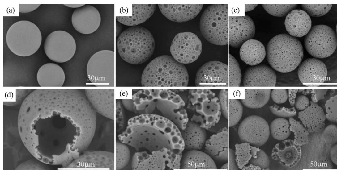
Fig. 1. SEM images of the PLGA microspheres: (a) non-porous MSs, (b) porous MSs, (c) hollow porous MSs, and (d–f) broken hollow porous MS.
